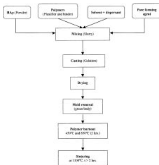
Figure 2 Controlled pore size HAp spheres formation through a modified gelcasting method.
